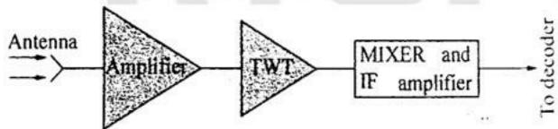
Gain  $Ga_1 = 30dB$   $Ga_2 = 20dB$   $Ga_3 = 40dB$ Noise Temp = 5°K Noise Figure = 6dB Noise Figure = 12 dB[6]
