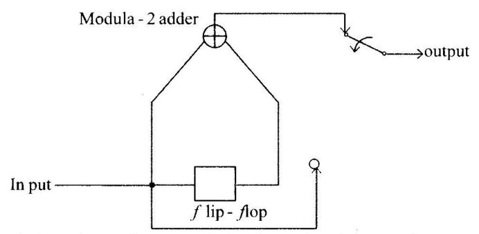
(b) Sketch the code tree for a convolutional encoder of rate r = 1/2. Constraint length K=2 given below:-
