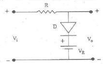
(b) Explain with an example positive peak clamping circuit with diode.
