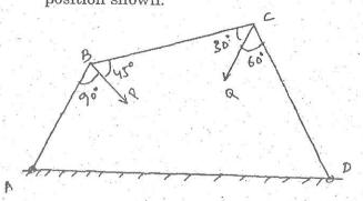
(b) Find the resultant of the following system of forces acting at a point:
