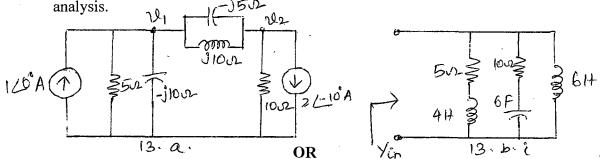
b.i). Determine the input admittance for  $\omega = 60$  rad/seconds in the circuit shown.
