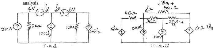
ii). Find  $v_1$  and  $i_2$  using nodal analysis in the circuit shown.
