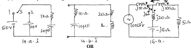
b. (i) Determine the value of L for which the circuit shown is resonant at 200Hz..
