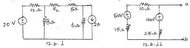
b.ii). Determine the power delivered to a 50  $\Omega$  resistor connected to terminals a and b of the circuit shown.
