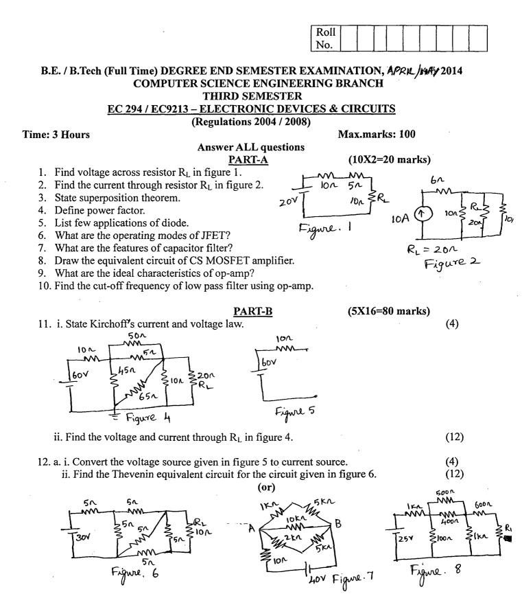
b. i. Find the resistance across A and B in the circuit given in figure 7 using delta to Y- (8) conversion.
