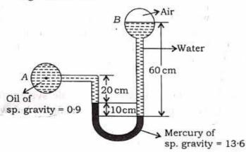
At B, air pressure is  $9.81 \text{ N/cm}^2$  (absolute), find the absolute pressure at A. 6+8=14
