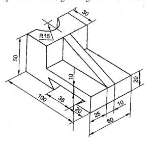
10) Draw the isometric view of the given figure. All dimensions are in mm.
